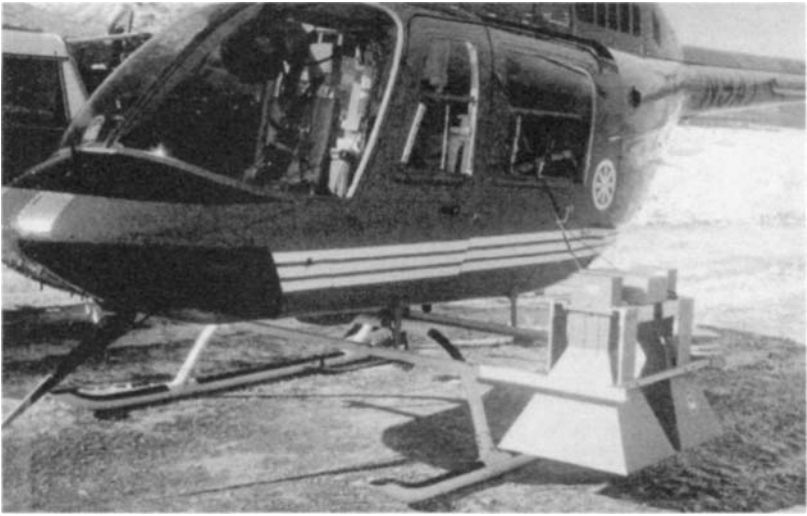
Figure 11.5 18 dB gain horn antennas for a 1–2 GHz FMCW antenna system
