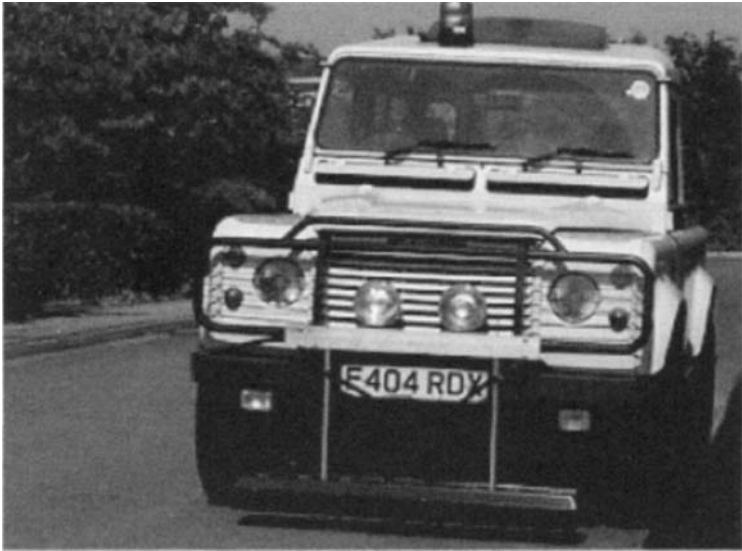
Figure 9.2 8-Channel, 1 m-wide experimental vehicle mounted radar system (courtesy ERA Technology)
