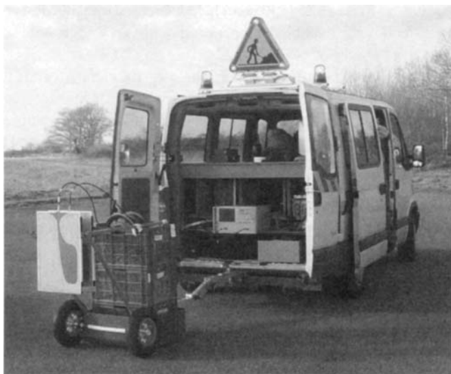
Figure 9.6 Step-frequency device in acquisition mode The network analyser and PC are on a truck; on the left are the Vivaldi-like antennas
