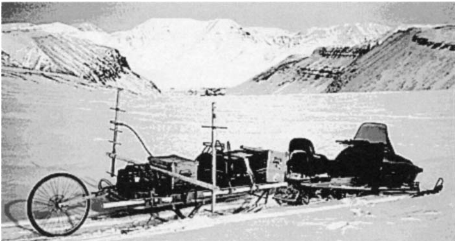
Figure 11.22 The photograph shows the radar set-up with UHF Yagi antennas and odometer wheel at the back
