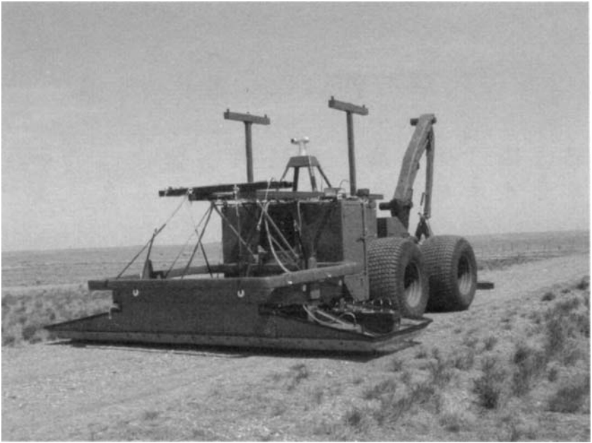
Figure 5.39 Photograph of downward look 32-channel array system used on MINDER system (courtesy ERA Technology)
