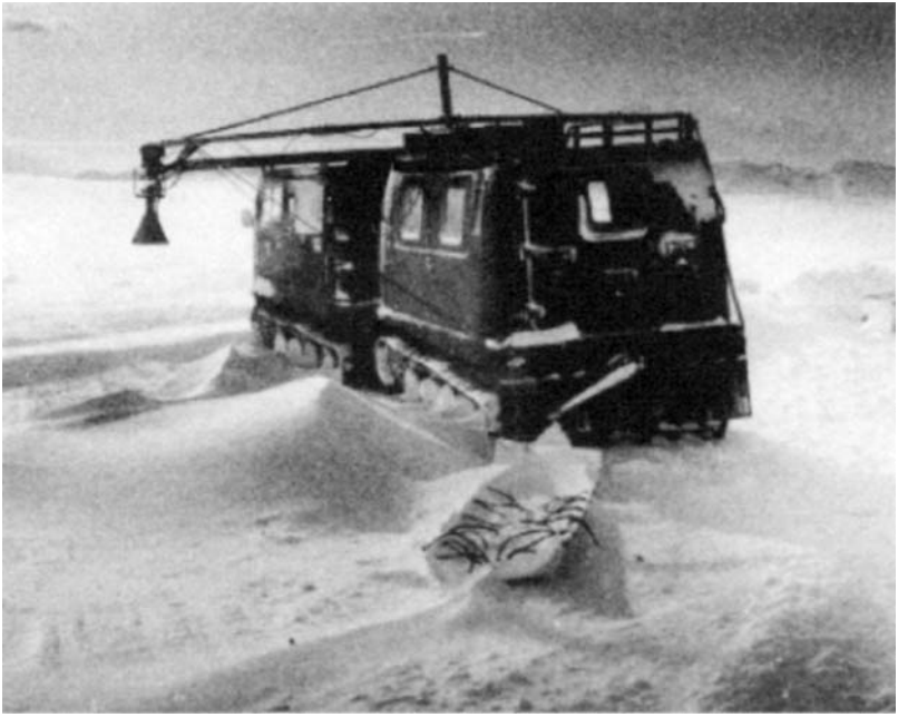
Figure 11.18 C-band (4–6 GHz) FMCW antennas mounted from a tracked vehicle travelling just south of Prudhoe Bay, Alaska
