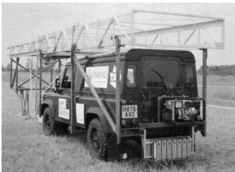
Figure 12.66 Rear of LOTUS vehicle showing paint marking system
