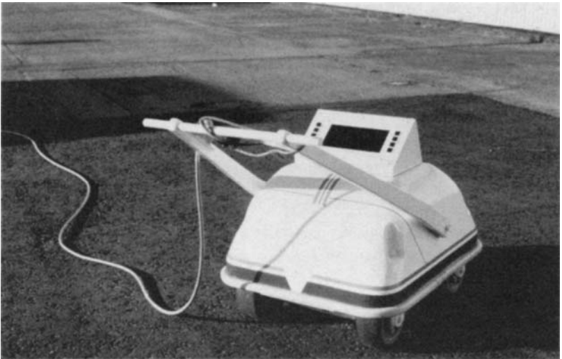
Figure 13.1 Radar head (courtesy British Gas)
