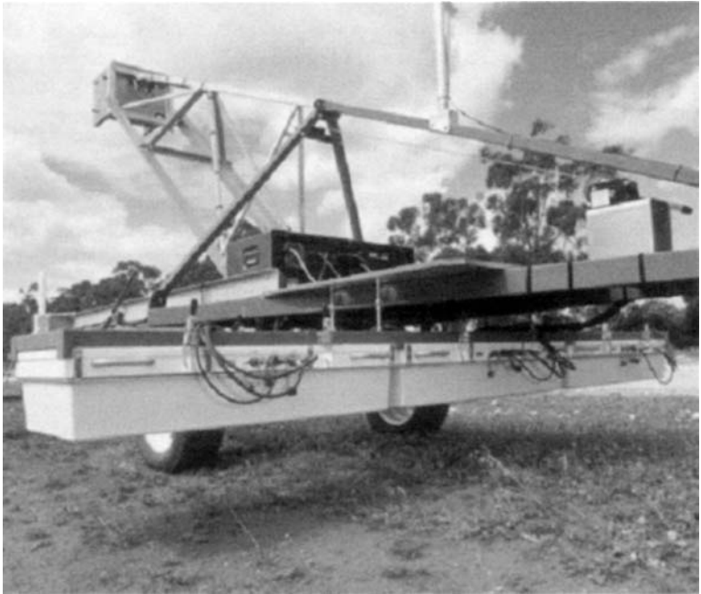
Figure 12.22 Three-metre-wide model 403 EFGPR arrays in initial testing at Australia's Defense Science and Technology Organisation (DSTO) (courtesy GeoCenters)
