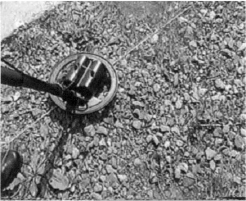
Figure 12.47 Photograph of MINTECT GPR antenna mounted on a Guartel MD
